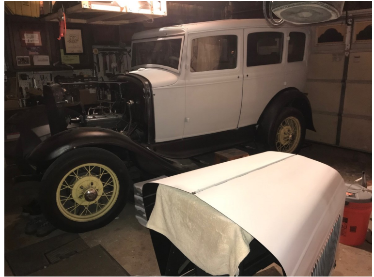
Nick Mazarella's 1931 slant 4-door reassembled, primed and ready for sanding over the winter in preparation for final painting next spring.
