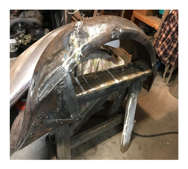
Nick's rear right fender is off the '31 slant 4 door . It was extensively damaged and corroded. Old rotted metal was removed and new metal was tacked into place in preparation for welding and brazing. The top of the fender has already been welded and then brazed for build up. Working on a fender off the car is tricky because the whole thing flops around like jelly. Mounting it on a saw horse helps stabilize it.
