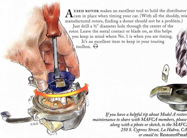
cam in place when timing your car. (With all the shoddy, mismanufactured rotors, finding a donor should not be a problem.) Just drill a ½" diameter hole through the center of the rotor. Leave the metal contact or blade on, as this helps you keep in mind where No. 1 is when you are timing. It's an excellent item to keep in your touring toolbox. O
