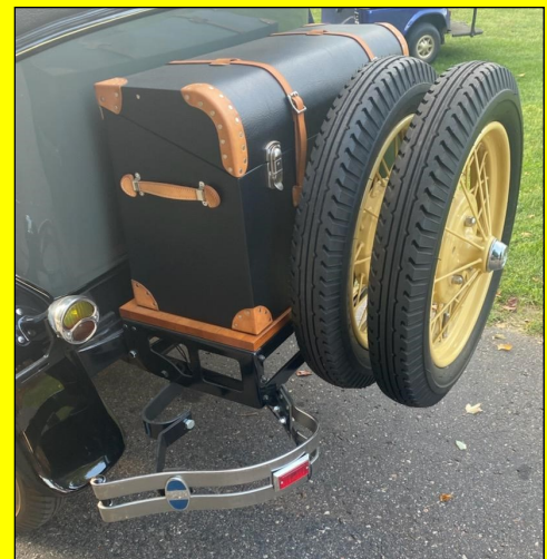
Double spare setup as mounted on a 1929 60B Model A, the Briggs "Leatherback" body style. Note the stationary trunk rack is inboard from the spare tire mountings.
