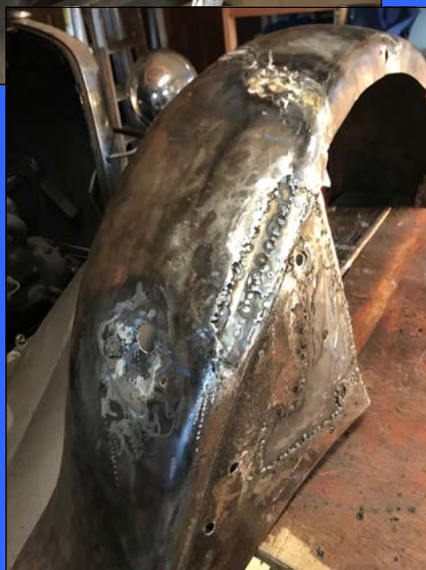
Fender parts being welded in, and, in some places, brazed to smooth out the welds. The seam on the top is a repair of a tear caused by a fender-bender collision several years ago.
