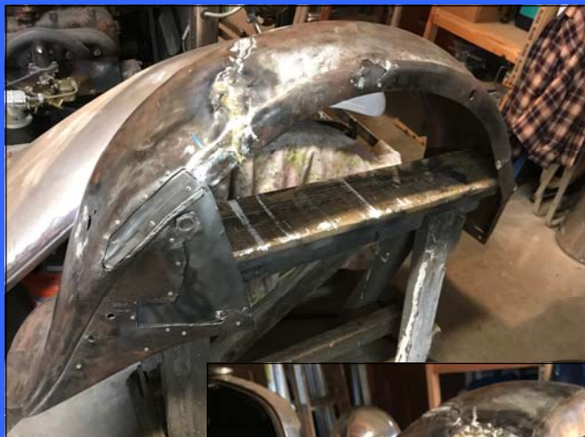
Start of adding new 22 gauge steel to the fender.
