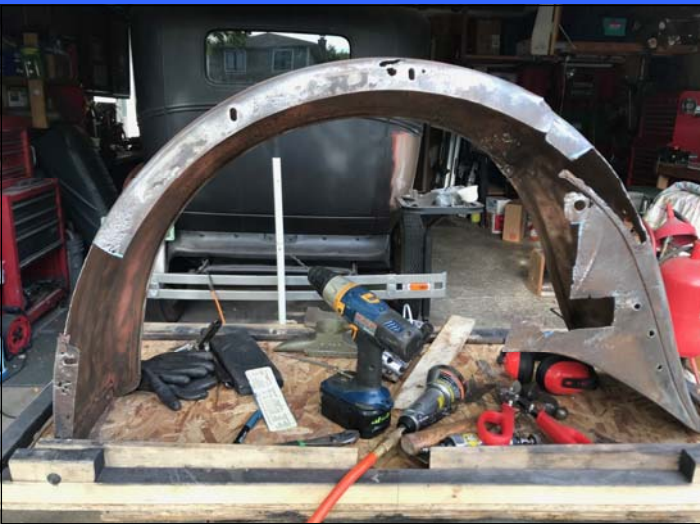
Fender after the rotted partitions were removed and a few tools of the trade.
