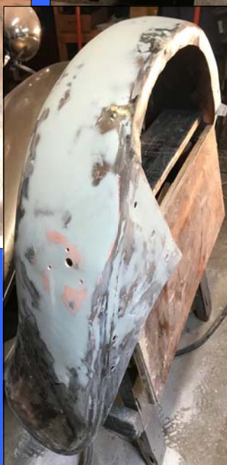
With the metalwork was completed, I applied filler compound to the reformed parts. These steps required a great deal of patience, diligence, and when finish sanding, plenty of elbow grease. I did not use glass or filler to cover any open holes, but only to even out surface irregularities and seal the welds. A good respirator mask was essential for this part of the process, as toxic vapor and dust are unavoidable when working with these materials. With glass and filler applied to smooth surface ripples, the fender was ready for priming. SEE PAGE ONE PHOTO FOR THE FINISHED RESULTS!
