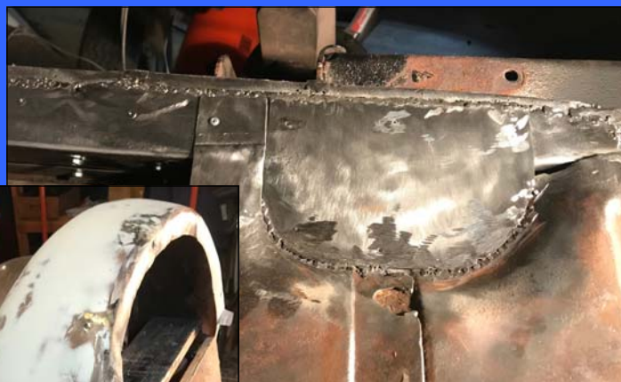
Panel rebuilding using individual 22 gage pieces to match the original stamped panel. Note that the nut plate the fender attached to needed new nuts welded in and then needed blending into the rear panel.
