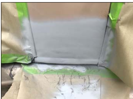
Photo 10: Driver's door lower corner welded and glassed.
