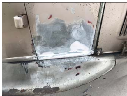
Photo 8: Right cowl welded and glassed.
