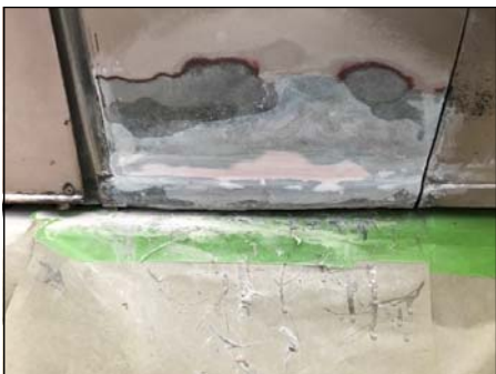
Photo 8: Right cowl welded and glassed.
