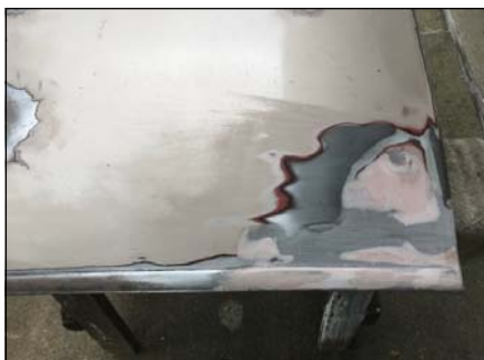
Photo 10: Driver's door lower corner welded and glassed.
