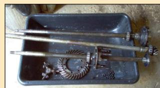
Differential parts and axles during cleaning and inspection.
