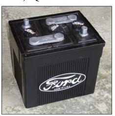
on How To Start Your Model A, fortunately revealing the Positive Ground issue and quickly resolving our mysterious problem. Yep, with the ground strap tied down on the <u>positive</u> battery post, she fired right up!
