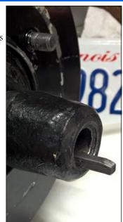
a little more than half way in (see photo). Carefully center the hub with the brake shoes and slide the hub onto the axle until it stops. Turn the hub from side to side until the key enters the mating keyway in the axle.
