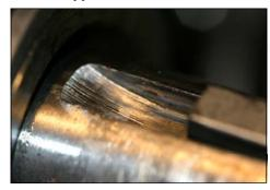
The problem is that the 1/4-inch key has moved into the rear keyway radius (see photo) and is not sitting at the bottom of the keyway. In other words, the key sits too high in the rear and won't let the hub taper seal against the axle taper.
