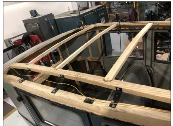
But no wood kit fits well without lots of measuring, cutting, sanding, and shaping the pieces to fit the car.
