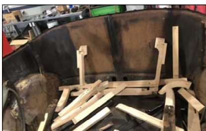
Badly rotted wood cannot hold the nails and screws that bind the top together.
