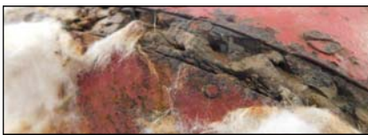
Badly rotted wood cannot hold the nails and screws that bind the top together.
