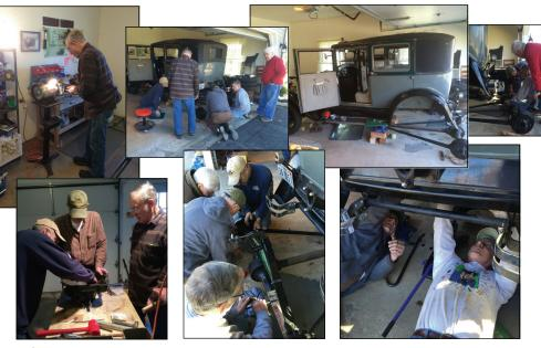
March 11th was a busy day in Paul Herbert's garage when Lindy, Ron, Gene, Fred, and Alan all came over to help put in a new clutch, pressure plate and throw-out bearing, replace the water pump, and re-install the rear end with a fresh rear spring that Ron had rebuilt. While Lindy was grinding away on a water pump shaft, heavy work was under way installing the rear end on Paul's 1929 Briggs Fordor Leatherback. Thanks to Gene and Alan for taking pictures!
