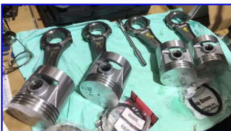
Pistons (EGGE Thin Ring, Made In USA) All Balanced, Matched Rods (All Within .5 Grams)
