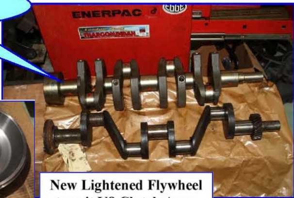
New 5 bearing crankshaft
