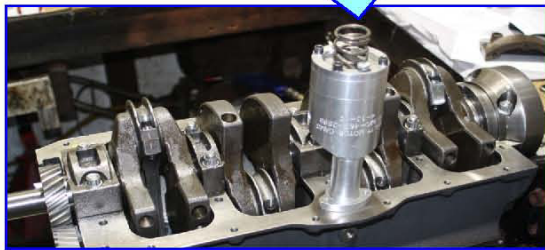
Pistons (EGGE Thin Ring, Made In USA) All Balanced, Matched Rods (All Within .5 Grams)
