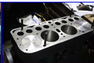
Pistons (EGGE Thin Ring, Made In USA) All Balanced, Matched Rods (All Within .5 Grams)
