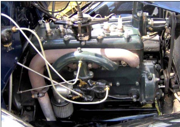
Original Air-Maze type installation, hanging down below the Zenith carburetor.
