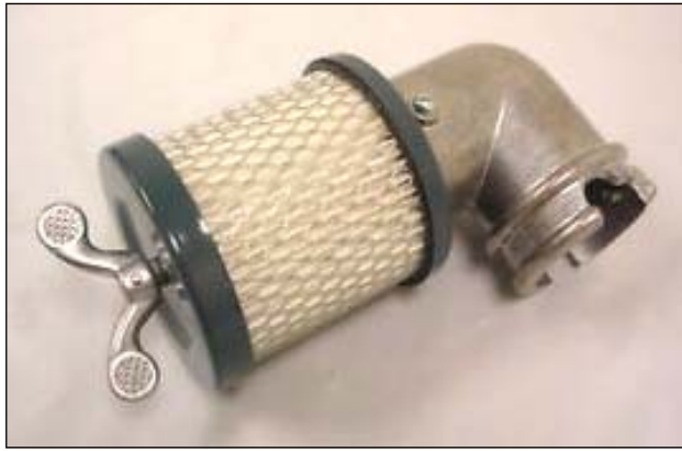
Air-Maze, as sold by vendors today with paper air filter element.
