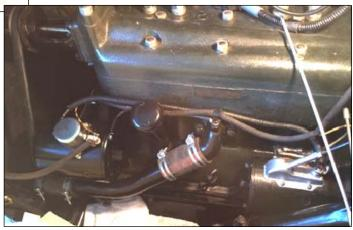
Belt installed and wiring additions complete. Note new #8 wires from generator to starter and to ground.
