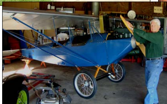
Gar acquired his 1930 Deluxe Coupe in 1959, while still in the service, adding the 1931 Deluxe Roadster and 1929 Town Sedan in later years. The Pietenpol "Air Camper" is an early 1930's homebuilt aircraft powered by a Model A engine adapted for aero use; here he demonstrates how the starter works.
